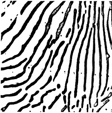
FIGURE 225. Metallographic structure of pearlite showing the relative thicknesses of the ferrite and cementite lamellae. Etched with saturated picral. \times 2500 , originally, reduced somewhat in reproduction. (Photomicrograph courtesy U.S. Steel Corporation Research Laboratories, Kearny, N. J.)
